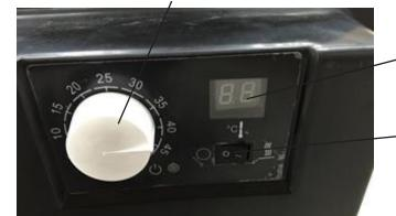
Digital Display (2% Tolerance with actual temperature)
